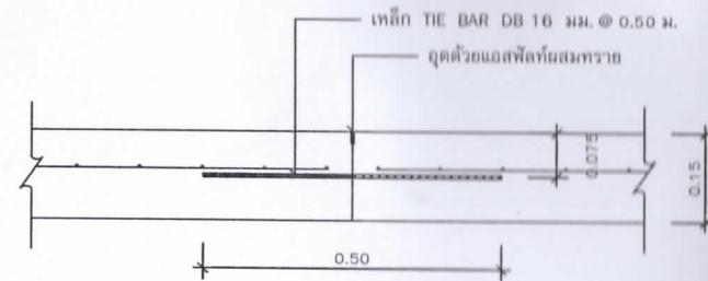
LONGITUDINAL JOINT SCALE _____ 1 : 10
